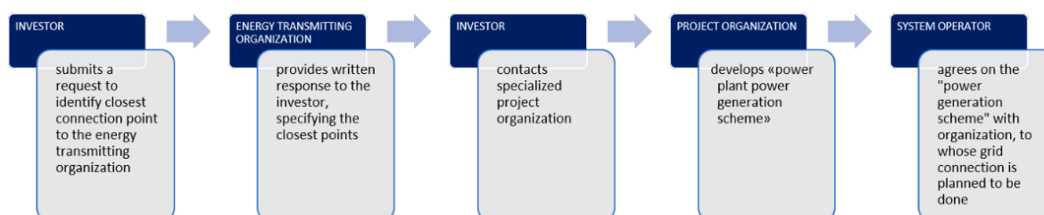
Figure 7. Procedure for Identifying the Closest Connection Point and Developing the Power Plant Power Generation Scheme
